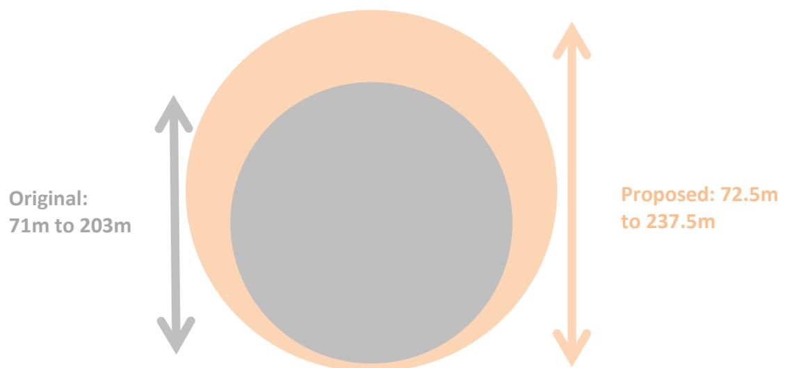
Figure 14. Indicative diagram of the original and proposed rotor swept areas. Not to scale.
